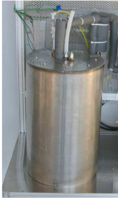
Fig. 1. Photograph of the 2.5 \text{ kW}_{\text{th}} compact steam reformer with separate PrOx as \text{CO} purification step in the test rig height: 600 \text{ mm} , diameter: 280 \text{ mm} .
